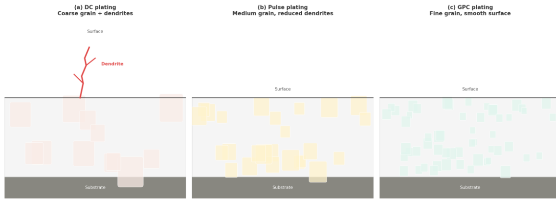
Figure 2. Grain structure and surface morphology: DC (coarse grain, dendrites), pulse (medium grain), GPC (fine-grained, smooth, dendrite-free). Schematic cross-sections.
